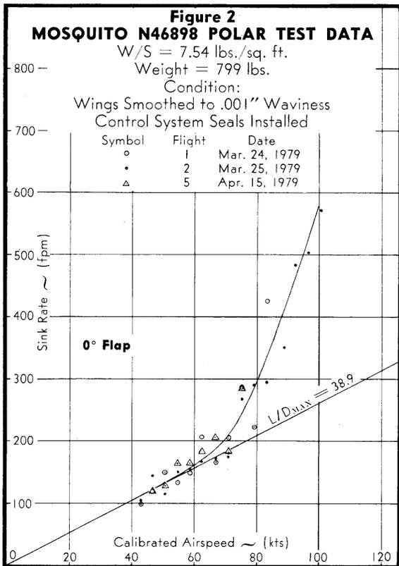
Mosquito had been filled and smoothed remarkably well by Alan Bikle about six months before our testing. My wave gage measurements could detect only about .001 inch peak-to-peak chordwise waviness, which is easily the smoothest wing that I have ever run my gage upon. Would this super smooth
