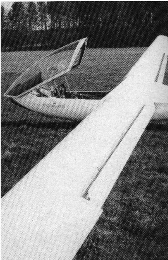
*Beyond 20° the upper surface airbrake begins to work in concert with the flaps, thus balancing the lower flap airloads and increasing the drag. "The system works beautifully; impressively steep landing approaches can be made with little practice," says the author.*
