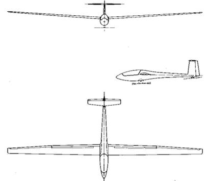
The Mosquito has very good stability and control characteristics, and it is very pleasant to fly. A fixed horizontal stabilizer combined with the excellent linked control-stick configuration provide outstanding longitudinal characteristics. Stalls are gentle and well mannered.
