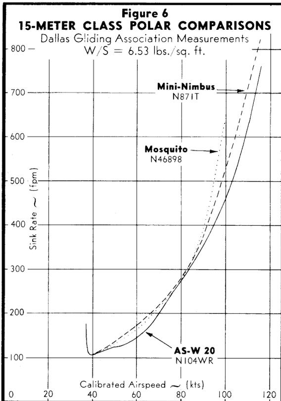
55 knots. The  $-7.5^\circ$  flap data in Figure 4 is less good scatter-wise, but with a little imagination it shows approximately the same polar as measured with the  $-4.6^\circ$  flap setting.
